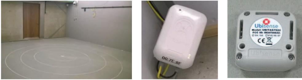
Figure 1. Test-room at Wageningen University (left panel), TrackLab beacon (middle panel), Active sending tag (right panel).
