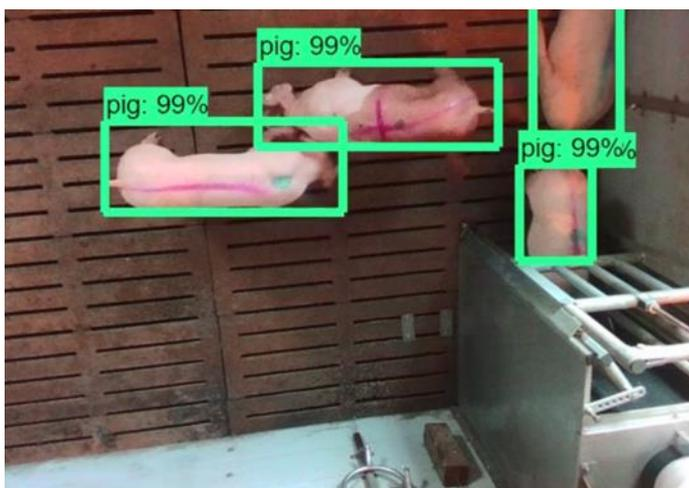
*Figure 1 - Results of detections of custom trained YOLO model*
